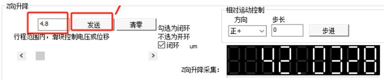
The screenshot shows the Z-axis control panel with the value '4.8' entered in the input field. The '发送' (send) button is highlighted with a red box. The '闭环' (closed loop) checkbox is checked, and the unit is set to 'um'.
