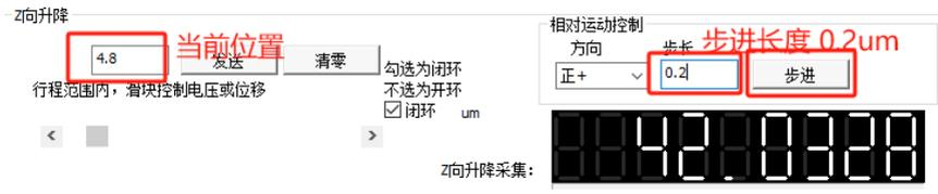
The screenshot shows the Z-axis control panel with '4.8' in the input field and '0.2' in the '步长' (step length) field. The '步进' (step) button is highlighted with a red box. Red text labels '当前位置' (current position) and '步进长度 0.2um' (step length 0.2um) are added to the interface.
