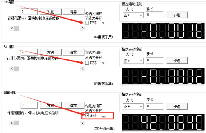
The screenshot shows three control panels for RX, RY, and Z-axis movements. Each panel includes a numerical input field, '发送' (send) and '清零' (clear) buttons, and checkboxes for '勾选为闭环' (select closed loop) and '不选为开环' (do not select open loop). The Z-axis panel also has a unit selector set to 'um' and a '闭环' (closed loop) checkbox which is checked. Red arrows highlight the '发送' button and the '闭环' checkbox in the Z-axis panel.
