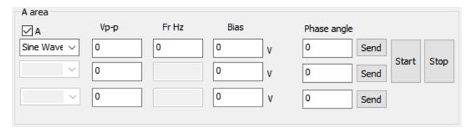
Fill in the corresponding data, click "Send" to send the data to the piezo controller, then click "Start" button to finish sending the phase angle waveform. Click "Stop" button to stop sending the phase angle function. Same goes for the other channels.
