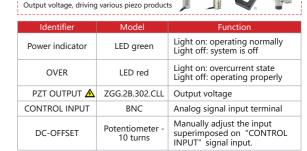
Note: Bipolar module has DC-OFFSET knob. If PZT OUTPUT or both ends of cables are directly measured through an oscilloscope and other instruments, when the output voltage exceeds 300V, pay attention to the measuring voltage range of the instrument to avoid damage to the measuring instrument!
